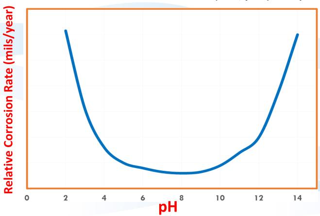
NB: Lowest relative aluminium corrosion rate at pH values between 7.5 and 8.5. Similar corrosion trend exhibited by other amphoteric metals such as zinc, tin.
